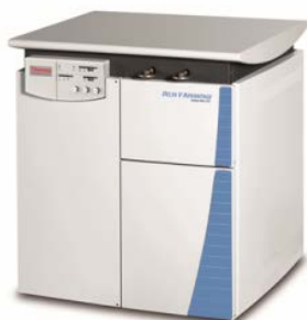
Figure 1.11: Thermo Scientific Delta V Isotope Ratio Mass Spectrometer and Dual Inlet standard performances
