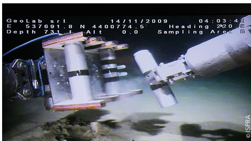
Sediment sampling with a ROV on the deep seafloor
