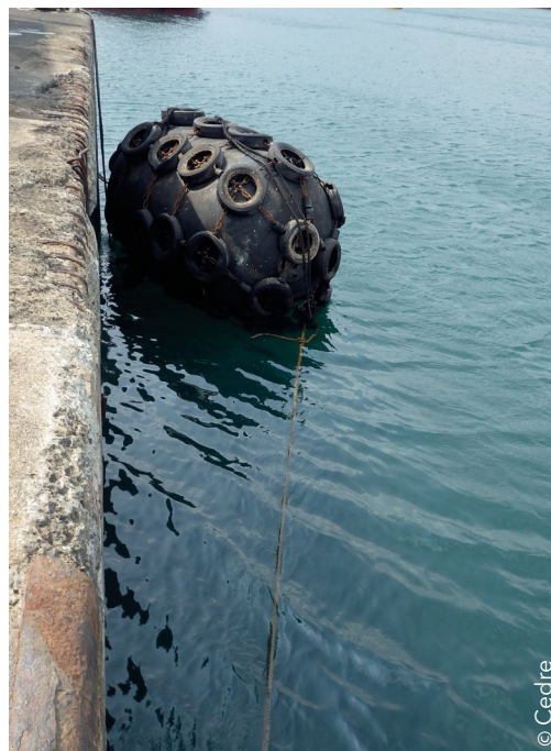
Yokohama fenders used to allow approach between two ships
