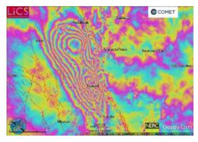
Figure 4: Interferogram of Sentinel-1 images acquired from ascending orbits before and after the earthquakes of 24.08.2016 (comet.nerc.ac.uk/) with faults (red lines) taken from the ITHACA catalog of the active and capable faults. Source: sgi.isprambiente.it/ ĞMV2/index.html
