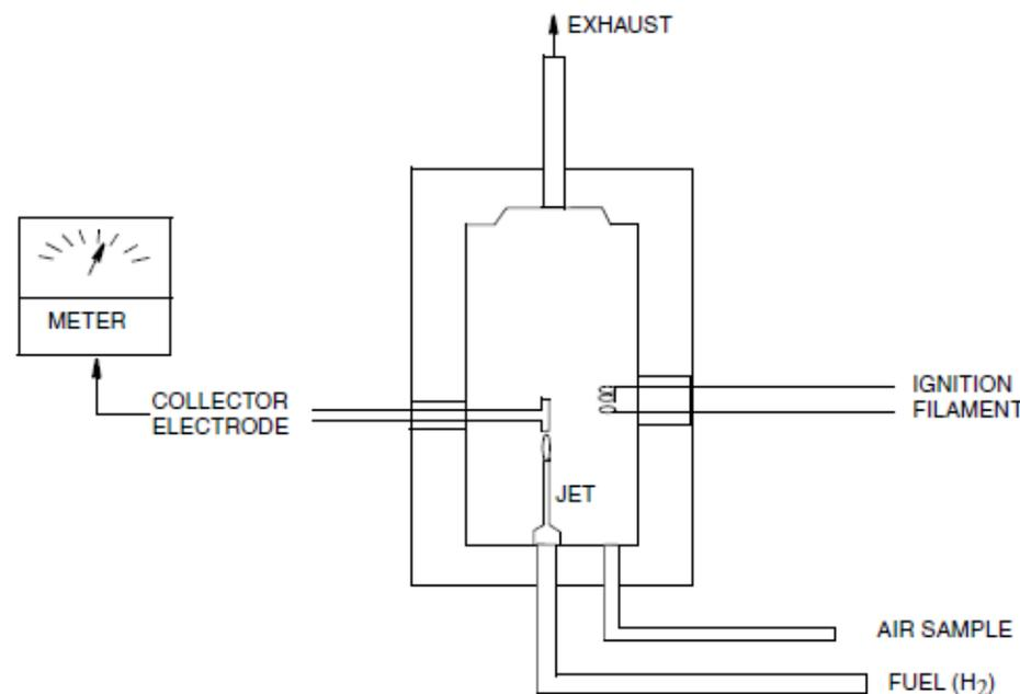
Figure 2. Typical Flame Ionization Detector
