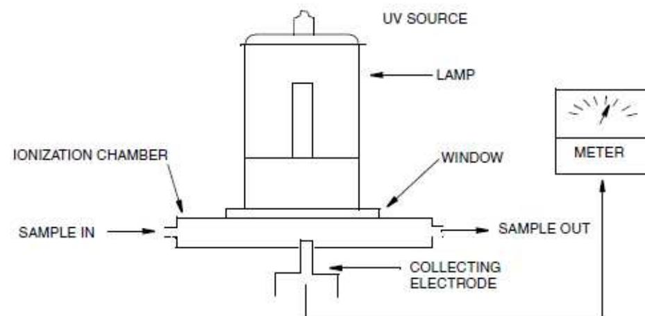
Figure 3. Typical Photoionization Detector
