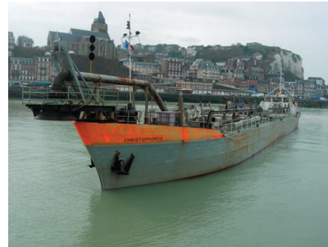
Suction dredger in the outer harbour of Le Tréport
