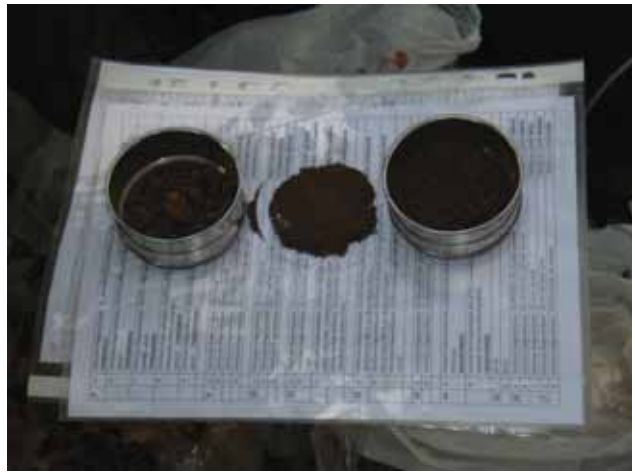
8) Sieves for the evaluation of the structure of the A zoogenic horizons.
