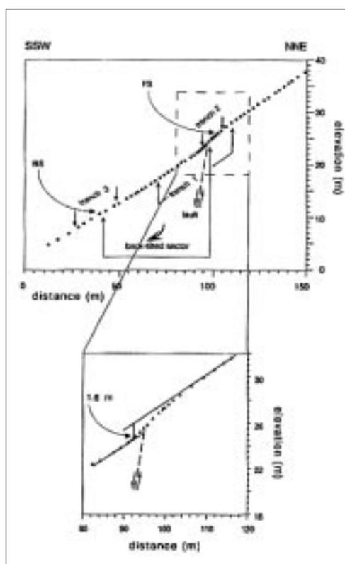
**Fig. 5.** Topographic profile at MQM (see location in Fig. 4); elevations relative to an arbitrary datum. Note the back-tilting of the alluvial fan deposits; no antithetic fault was found in trench 3, dug across its lower boundary (BS). The vertical displacement of 1.6 m across the main fault scarp (FS) is therefore greater than the net vertical tectonic offset at this site.
