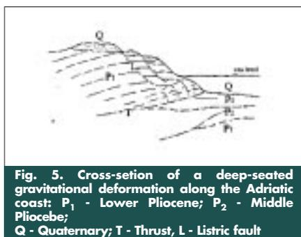
Fig. 5. Cross-section of a deep-seated gravitational deformation along the Adriatic coast: P<sub>1</sub> - Lower Pliocene; P<sub>2</sub> - Middle Pliocene; Q - Quaternary; T - Thrust, L - Listric fault
