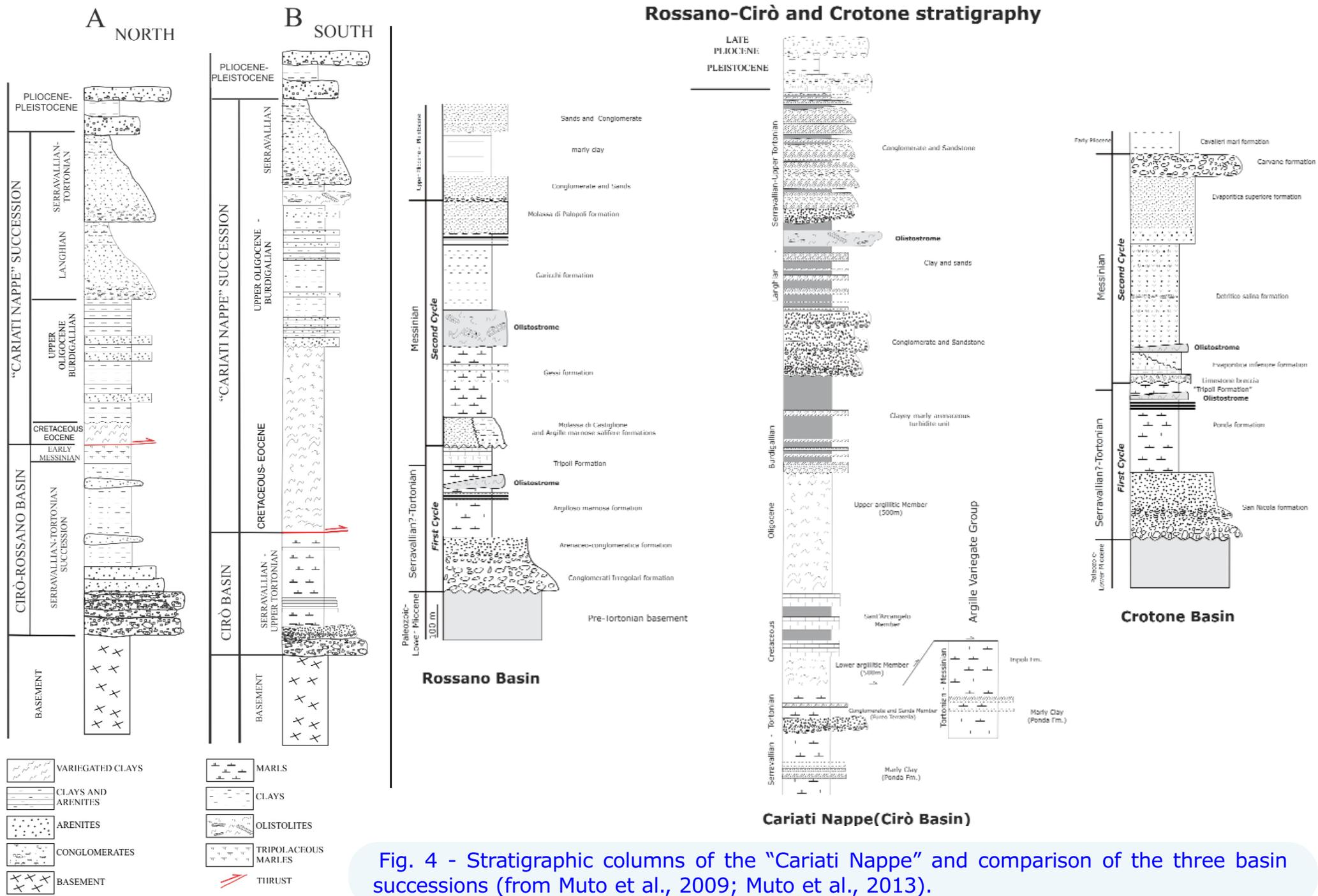
Fig. 4 - Stratigraphic columns of the "Cariati Nappe" and comparison of the three basin successions (from Muto et al., 2009; Muto et al., 2013).
