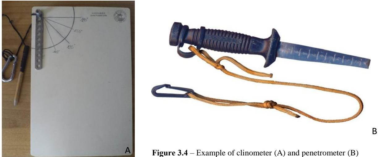
**Figure 3.4** – Example of clinometer (A) and penetrometer (B)
