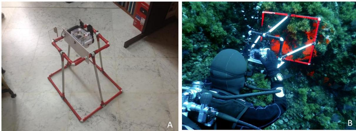
**Figure 3.1** – Example of a pvc frame with fixed surface and spacer (A) and its use in the field (B)
