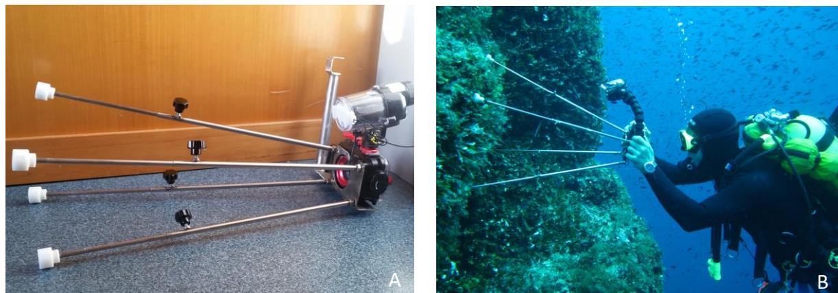
**Figure 3.2** – Example of a stainless steel frame with adjustable surface and spacer (A) and its use in the field (B)
