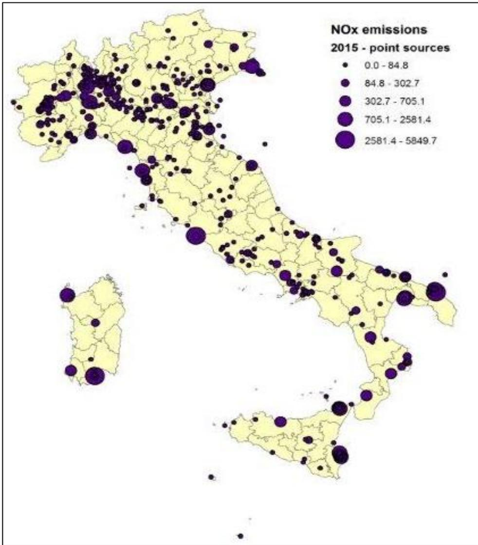
In Figure 3.3, NO<sub>x</sub> emissions communicated by 229 facilities (power plants, refineries, cement plants and iron and steel integrated plants), in the framework of the national E-PRTR register and LCP Directive, have been processed and geographically located. The territorial distribution shows similar results to those reported in the previous figure highlighting the industrial areas still in activity in 2010.
